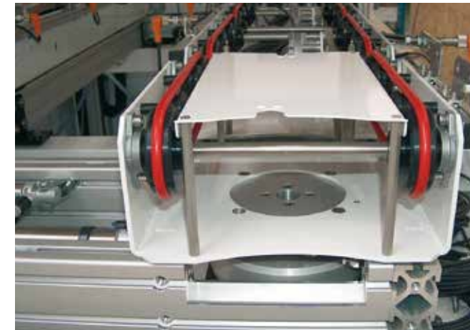
iglidur® PRT-01-60 is used here in a handling/transport system for semiconductor carriers. Through a cylinder control, the PRT polymer slewing ring bearing provides a deflection at the end of the system's track.
