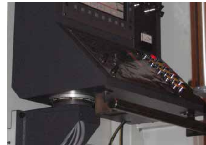
In this machine tool control panel, an iglidur® polymer slewing ring bearing is used due to its freedom from lubrication and maintenance.
