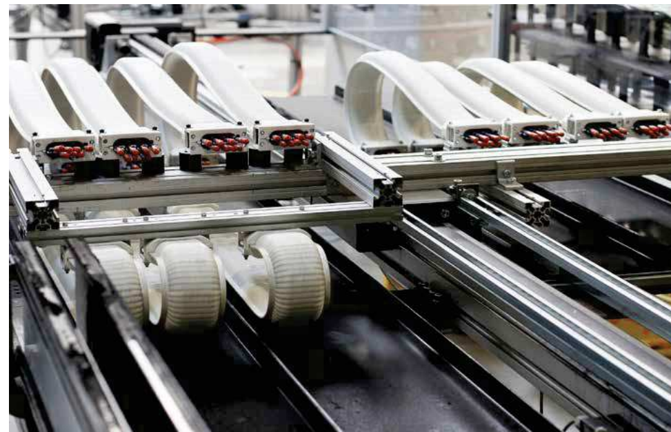
Service life test in the 3,800m² igus® laboratory in Cologne (Germany)
