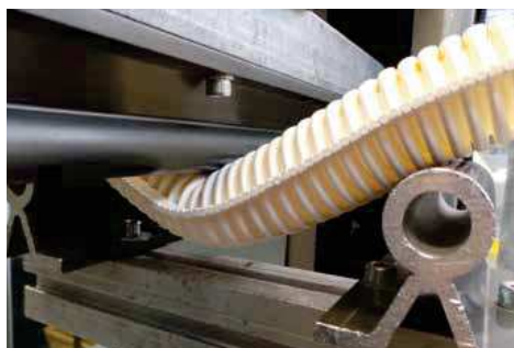
The standard bending tests show how flexible the e-skin® soft is. It only bends, even under loads that would break other energy chains
