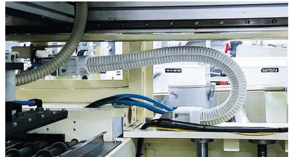
Absolutely dust-free environment for printed circuit board production using the abrasion-resistant e-skin® from igus®
