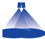
TwinAbsorbPRO Equilateral full cone
