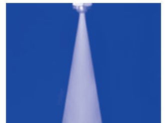
Spray pattern of the Laval nozzle
