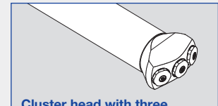
Cluster head with three nozzles with barrier air Spray width approx. 55°, spray depth approx. 15°; flat fan
