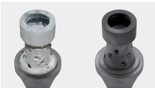
A visible difference: nozzles before and after LOC automatic cleaning
