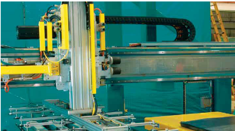
A linear drive provides the highly dynamic feed for PCBs. This system is twice as fast as handling units with a toothed-belt drive; designed to withstand high dynamic loads, E6 e-chains® ensure a supply of power, coolant and control data with ultra-low noise and vibration
