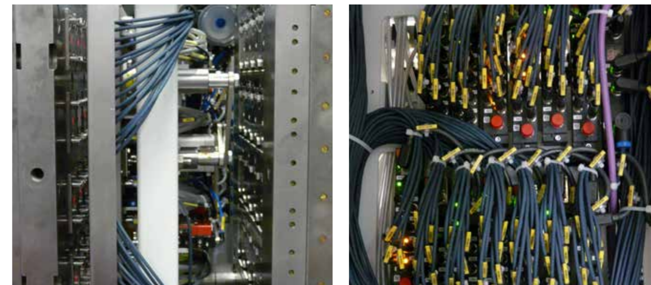
chainflex® CF9 INI cables in a high-performance system for plastics processing with cycle times in seconds. e-chain® E6 series. (Source: Hekuma)
