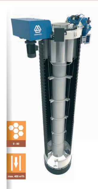
Telescopic loading spout type NZOF400E with the powerful built-in filter, dustproof bell with rubber skirt and level indicator guarantee you a dustless loading of dry, dusty bulk solids on trucks or railway cars.
