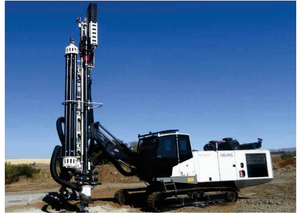
igus® E4.1 in an earth drilling machine. Standing installation, it defies strong vibrations. Thanks to plastic, no loose parts such as rivets or screws
