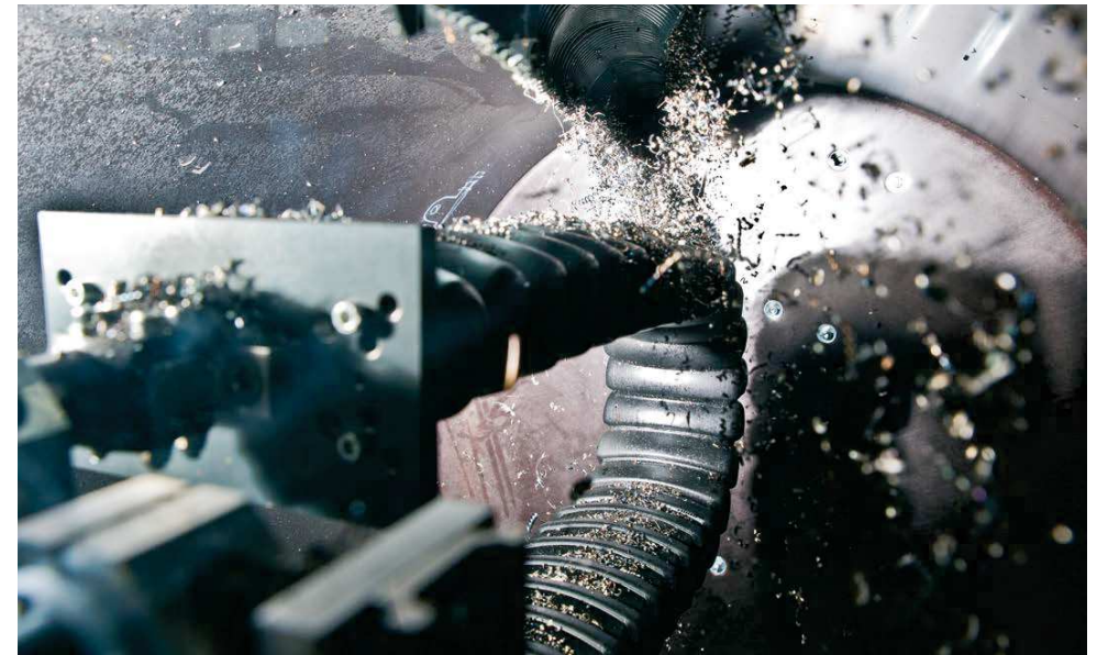
Swarf tests at the igus® test lab prove the excellent sealing of igus® RX e-tube. Video online ► www.igus.co.uk/RX_tested
