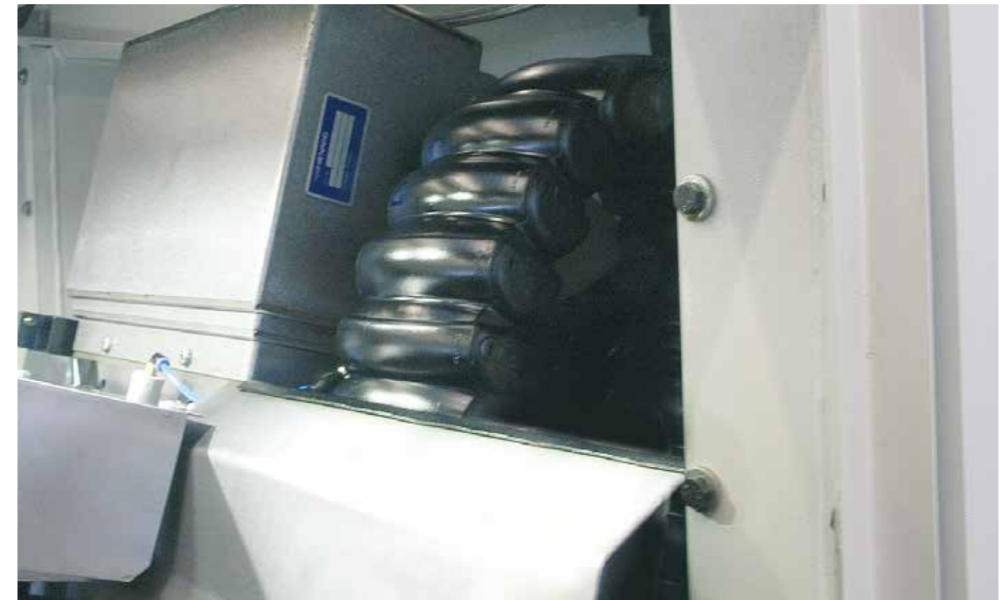
The RX e-tube used in this compact turning machine has Reverse Bend Radius (RBR) and operates even with the very restricted space
