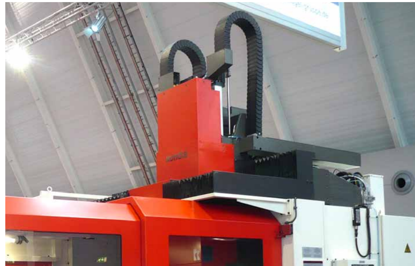
Typical use of igus® E2 R100 e-tubes - standing application in a machine tool
