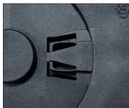
Special brake in the stop-dogs reduces noise level by up to 3dB(A)
