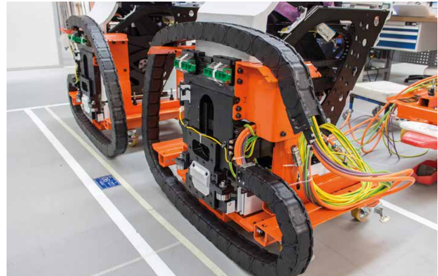
The R4.1L e-tubes are used to guide motor, encoder and sensor cables to supply the moving part of this bending machine
