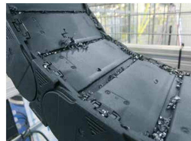
Swarf test in the igus® lab - protection proven in this test; stop-dogs completely free of swarf
