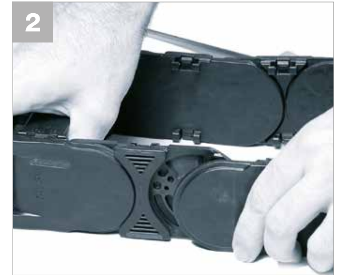
... insert the undercut of the outer link into the groove on the inner link and click together
