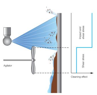
Figure 5: Cleaning mechanisms, impact and shear stress
