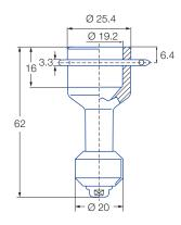
**Dimensions slip-on connection** according to ASME-BPE (OD-tube)
