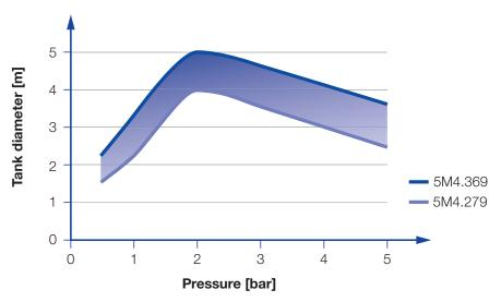
Overview of the tank diameter, depending upon the pressure of series 5M4
