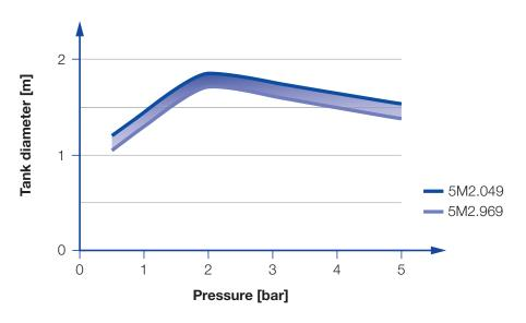
Overview of the tank diameter, depending upon the pressure of series  $5\mbox{M2}$
