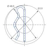
**Dimensions** slip-on connection top view
