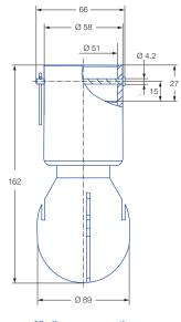
1 1/2" slip-on connection Dimensions slip-on connection according to ASME-BPE (OD-tube)
