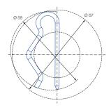
3/4" Slip-on connection Dimensions slip-on connection according to ASME-BPE (OD-tube)
