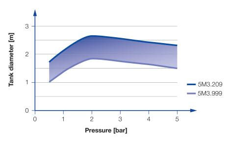
Overview of the tank diameter, depending upon the pressure of series 5M3
