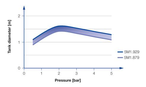
Overview of the tank diameter, depending upon the pressure of series  $5\mathrm{M}1$
