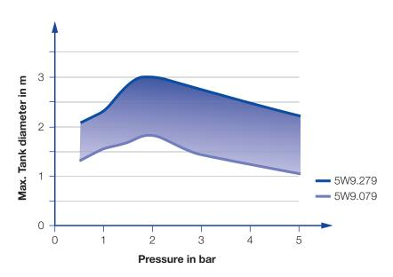
Overview of the maximum tank diameter, depending upon the pressure of series 5W9
