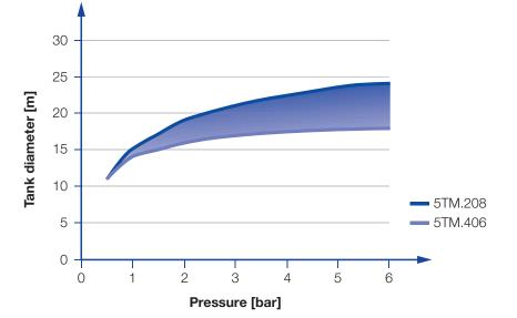
Overview of the tank diameter, depending upon the pressure of series 5TM
