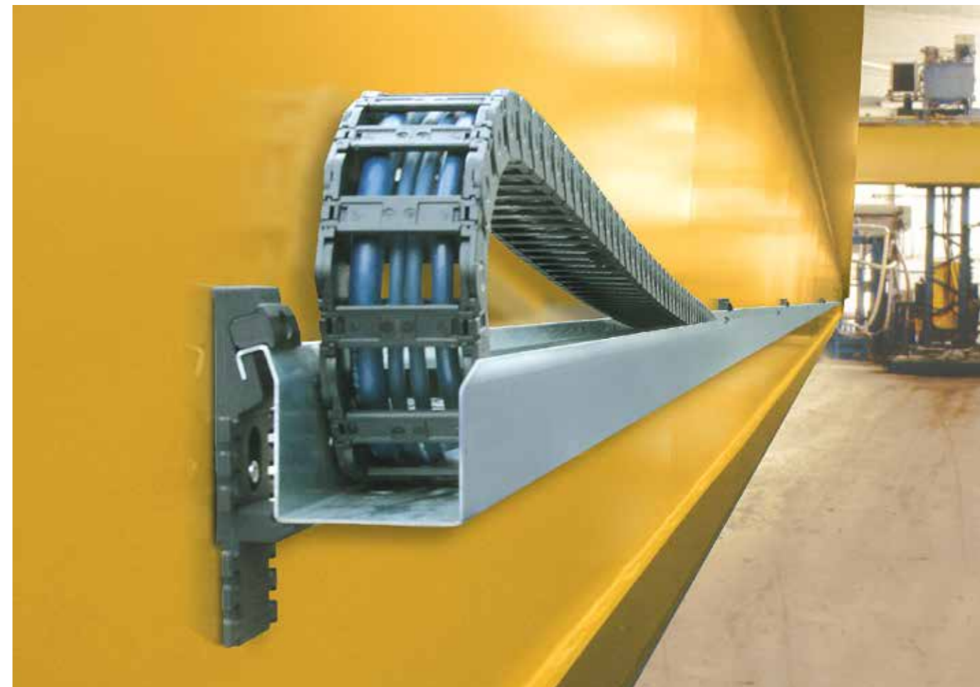
guidefast - easy attachment to the crane girder using welded bolts or nut/thread, here with version 2 long trough bracket
