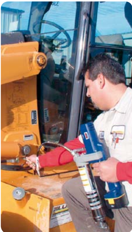
BDS bearing dosage system for lubricating connected lubrication points through one single inlet
