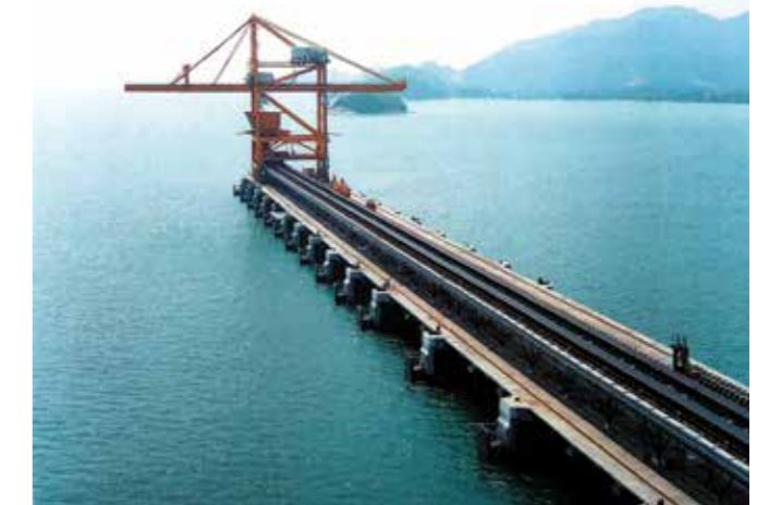
Cross travel of 441.3m, implemented with igus® E4/4 rol e-chain® series 5050R
