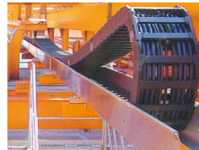
igus® E4/4 rol e-chain® saves drive power on long travels. Safely guided in igus® guide troughs
