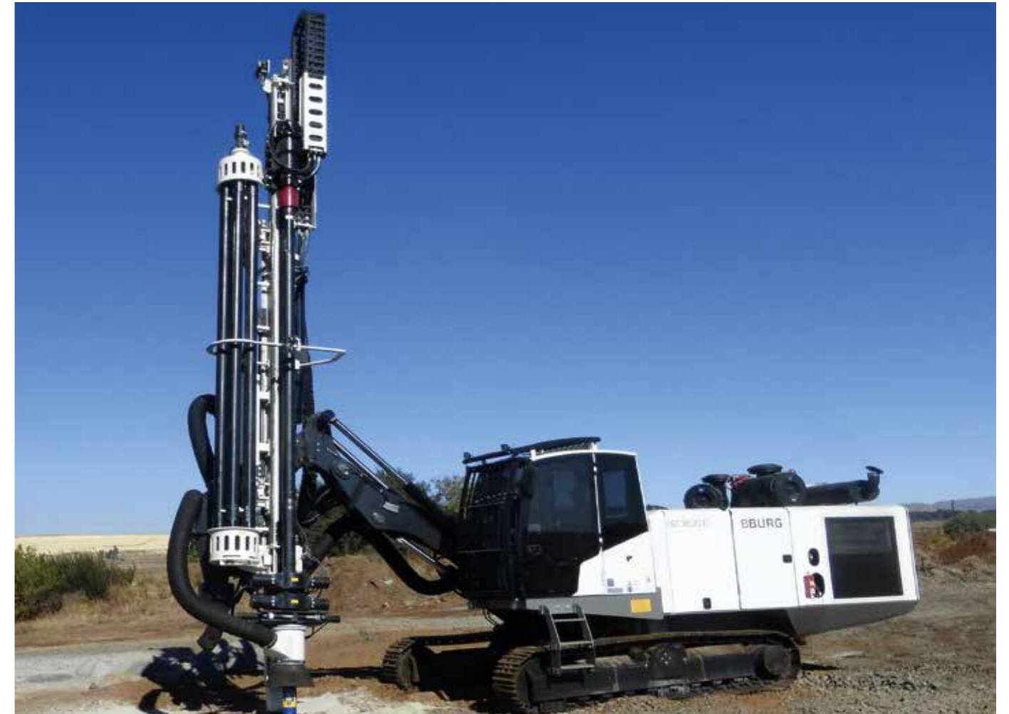
igus® E4.1 in an earth drilling machine. This vertically standing installation works even under strong vibration and harsh environments due to its plastic construction and having no loose parts such as rivets or screws
