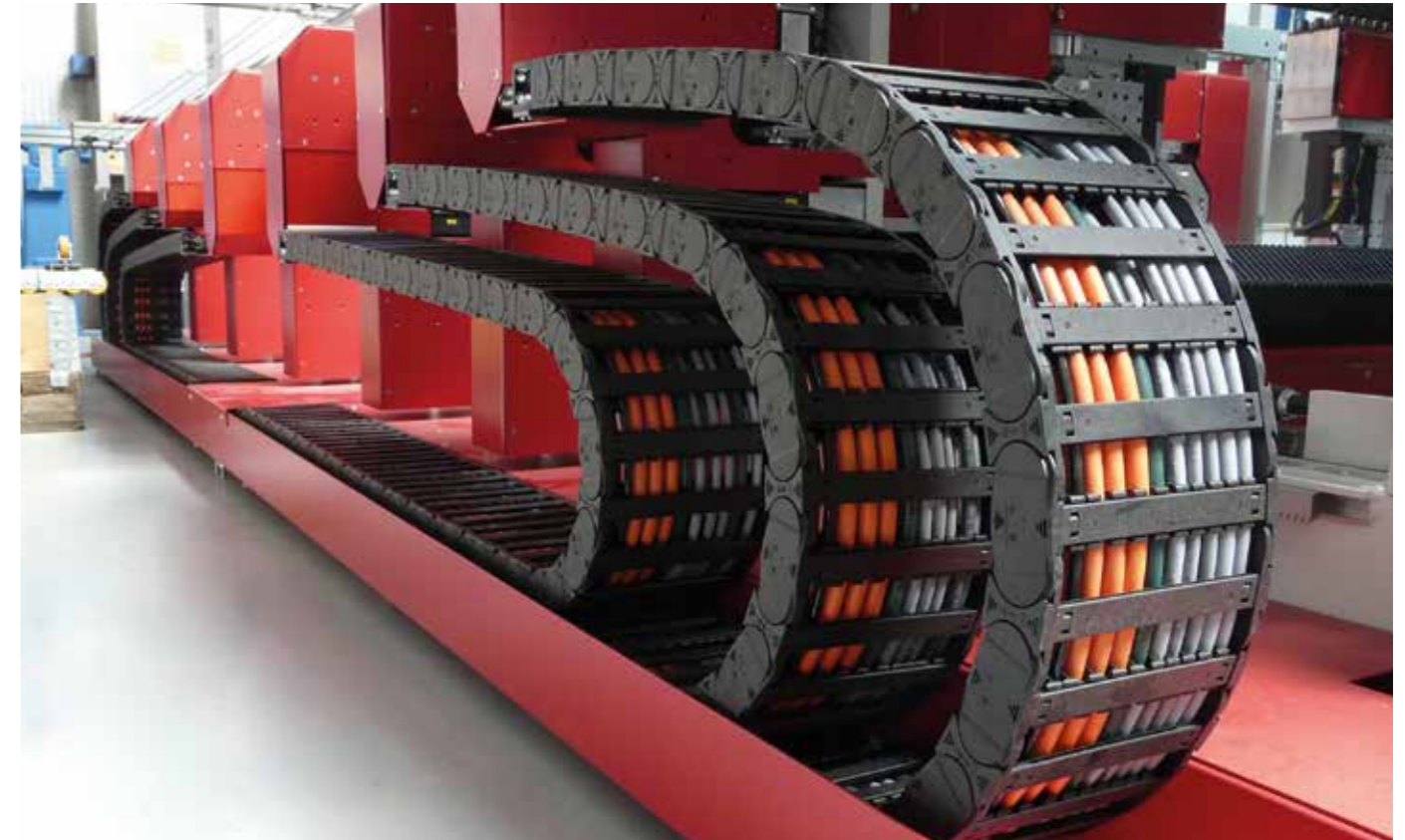
E4.1 e-chains®, supplied as readychains®, reliably supply power and data to different axes of this machine tool
