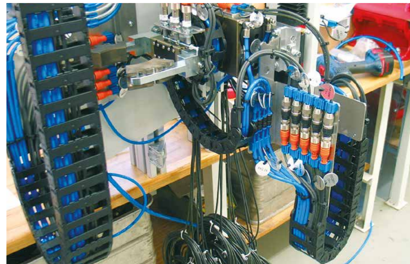
E2/000 - dirt-resistant e-chain®, which saves installation space - here in a machine tool for workpieces
