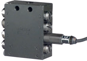
SSV8 N with piston detector
