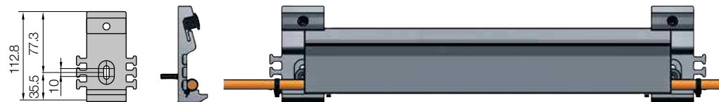
Version 01 - short trough bracket Part No. GF9.2.12 with integrated strain relief, ± 5mm vertical adjustment (electrically conductive version: GF9.2.12.CD)
