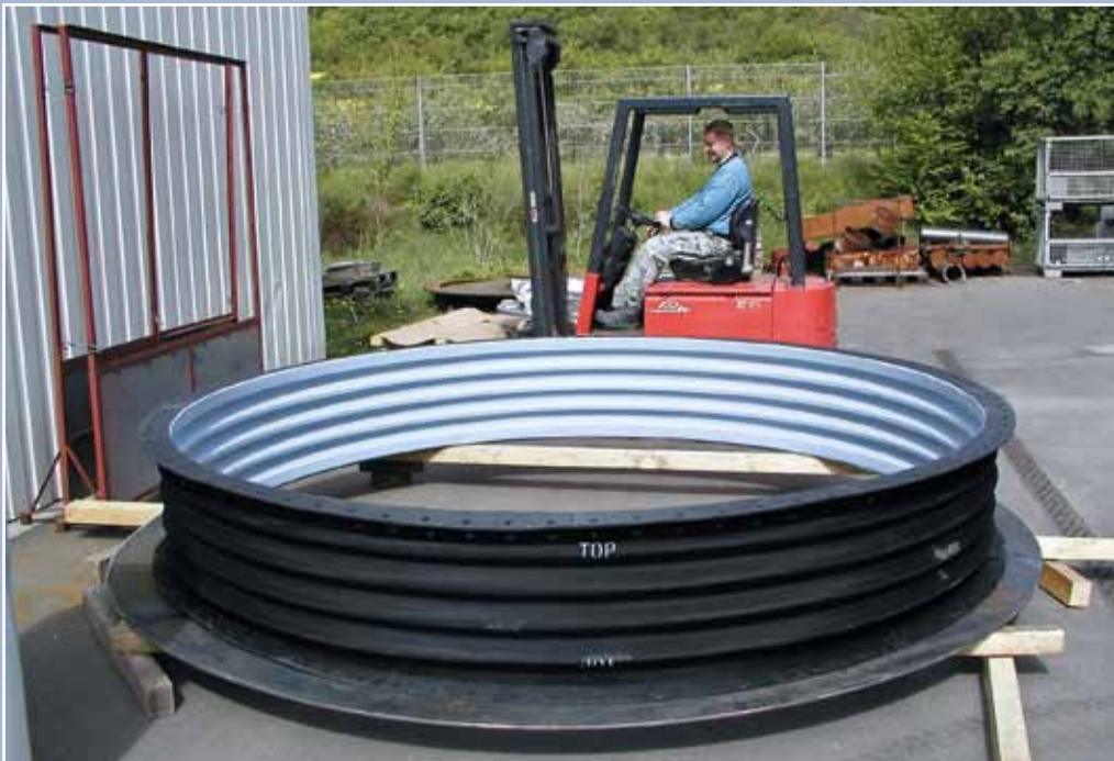
Universal expansion joint, type U142A with PTFE lining for a sulphuric acid reclamation plant NB 2800, -0.15 bar, 80 °C
