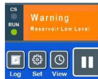
Early warning of potential failures with full text display provides possibility to take preventive action
