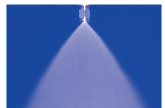
Spray pattern of a single spillback nozzle
