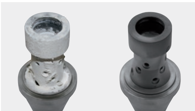
A visible difference: nozzles before and after LOC treatment
