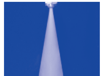
Spray pattern of the Laval nozzle
