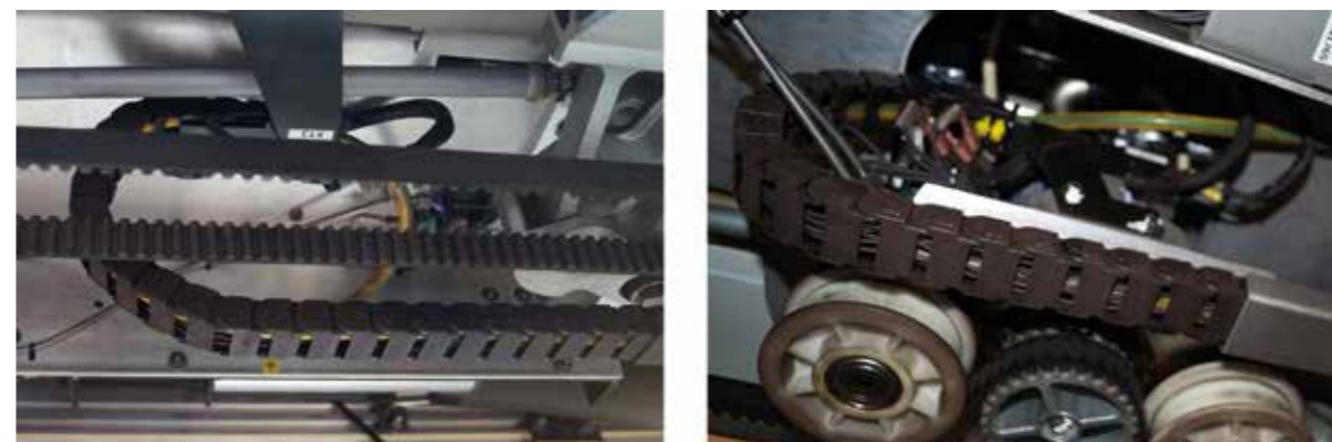
chainflex® CFSPECIAL.414 in automatic door systems for underground railway vehicles of VAG Verkehrs-Aktiengesellschaft Nürnberg, each approx. 70,000 opening and closing cycles per year. e-chain®: E2 micro series.
