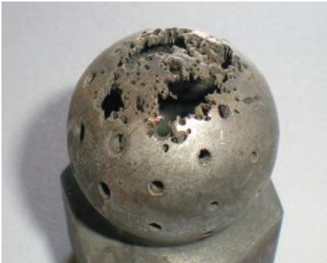
Figure 13: Chemical attack on a spray ball
