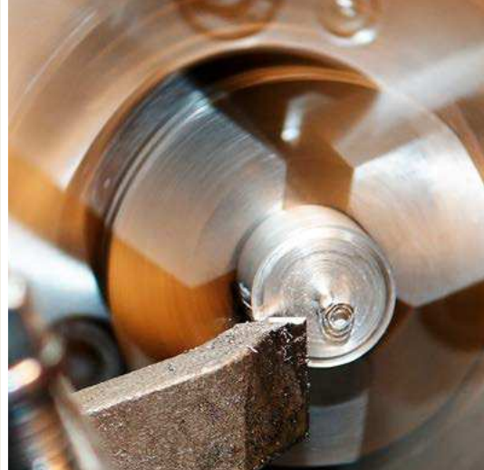
Counterbores for solderless tube connection (DIN 3854/DIN 3862)
