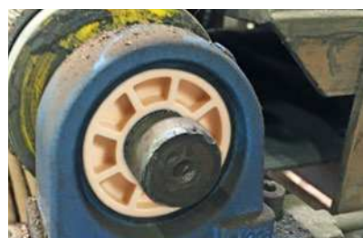
Top: igus® tribo-tape in desired shapes Bottom: igubal® bearing inserts
