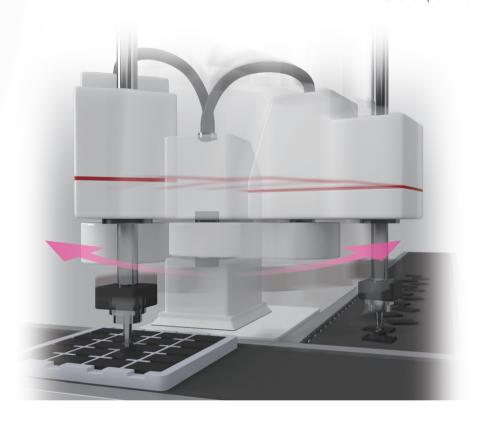
Customers are looking for low-inertia Z axes to improve the takt time of horizontal articulated robots.
