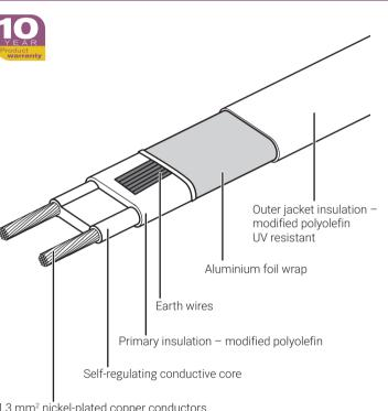
The nVent RAYCHEM BSA self-regulating heating cable is designed for industrial pipe freeze protection without steam cleaning and moderate process temperature requirements. It can be used for indoor and outdoor installation in ordinary (non-hazardous) area applications.
