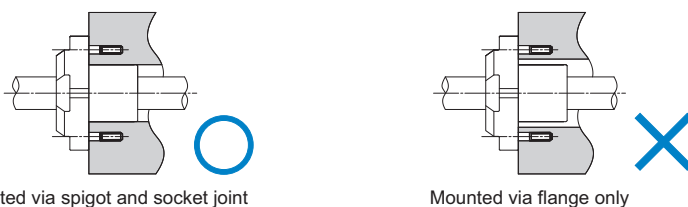
Mounted via spigot and socket joint
