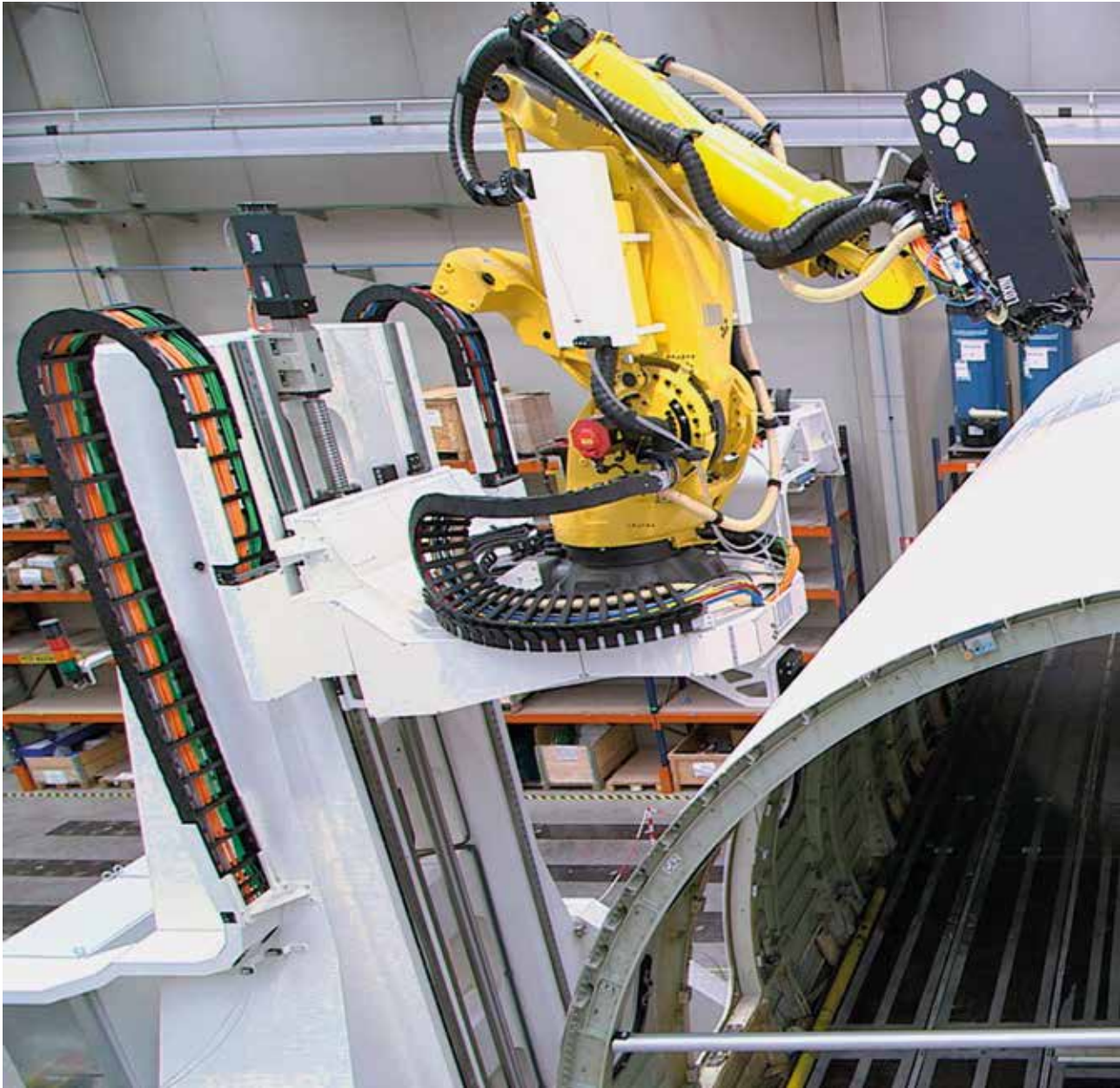
chainflex® servo cable in a vertical e-chain®
