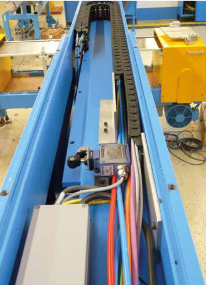
Adjustment device with chainflex® CF898 bus cables
