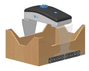
By increasing the finger height, the allowed torque might be reduced as shown in the **Moments in the finger base** section.
