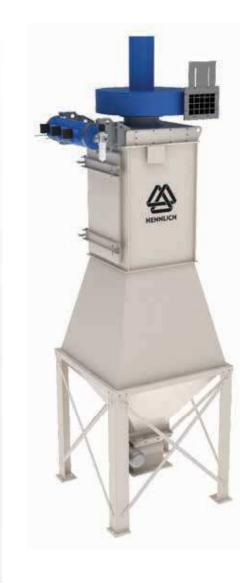
Dust collector type P1500/9/R with the support frame and rotary valve is used for the local filtration – dedusting of big-bags filling, welding and cutting machines etc.
