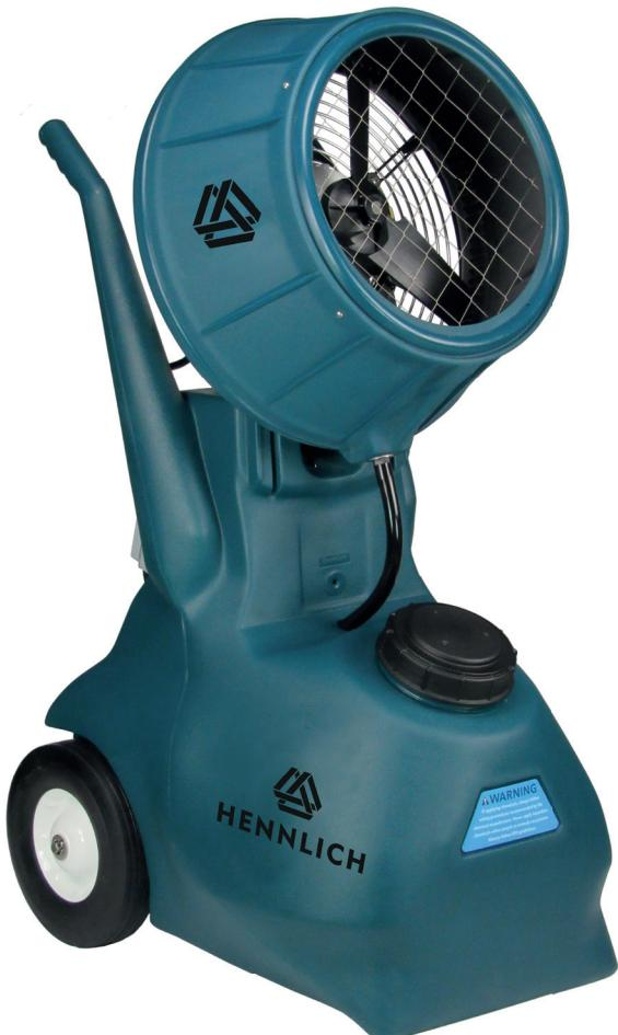
The mobile fogger HE-ORSM combines the powerful fog fan with a large water tank designed for mobility and ease of use. The tank captures and recycles wastewater and can be used in chemical fogging. Centrifugal atomization produces billions of tiny, fog-like particles that quickly evaporate. The fogger uses a float valve to maintain the water level, a submersible pump to feed the fogging head, and ball valve to control the fogging output.
