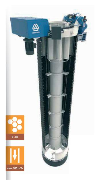
Telescopic loading spout type NZOF500E with the powerful built-in filter, dustproof bell with rubber skirt and level indicator guarantee you a dustless loading of dry, dusty bulk solids on trucks or railway cars.
