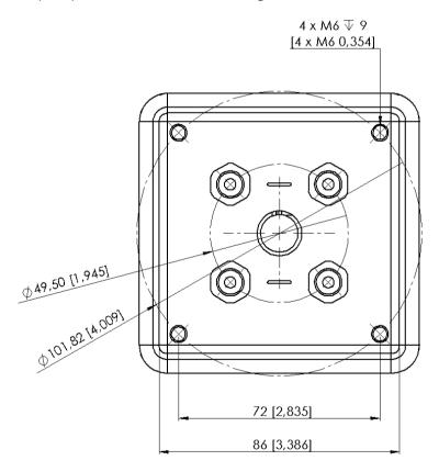
The Push-in Fittings are used to attach 4 mm vacuum tubes to create customized configuration that required remote vacuum. In most cases, this size is enough for generating the needed vacuum from the pump in the gripper.
