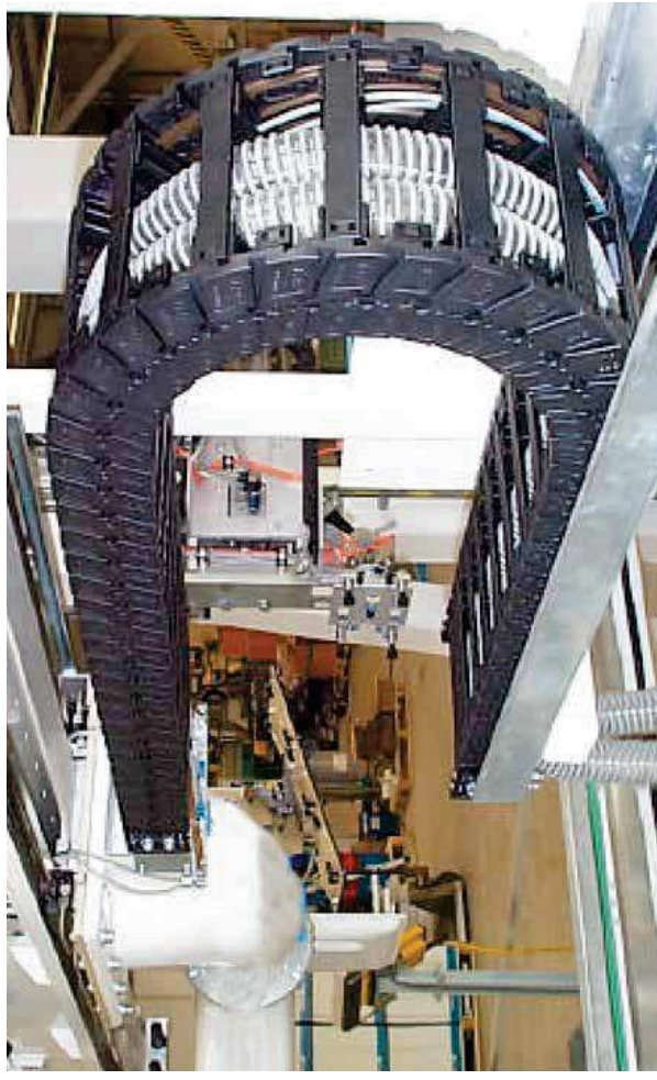
igus® system E6 guiding an extraction hose - speed 8m/s, acceleration 78.5m/s 2
