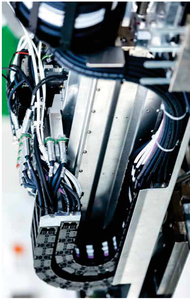
Cleanroom suitable E6.1 series as a harnessed readychain® system for the semiconductor industry
