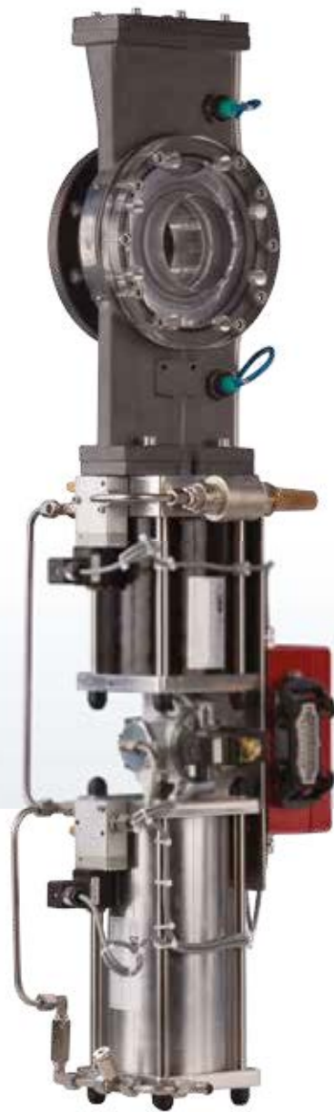
Fast-closing valve: closes within milliseconds
