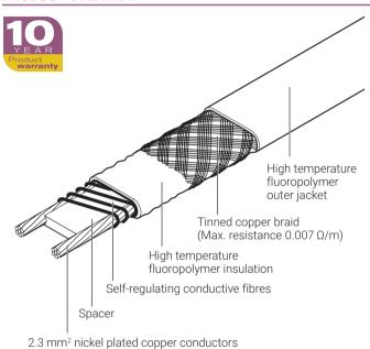
Electrical heat-tracing for process temperature maintenance applications up to 150°C which may be subject to steam cleaning.
