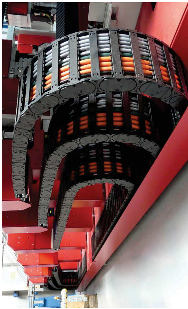
E4.1 e-chains®, supplied as readychains®, reliably supply power and data to different axes of this machine tool
