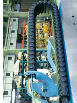
Supply of the main spindle in a tooling machine with igus® RX e-tube. The rounded contour of the energy supply repels all kinds
