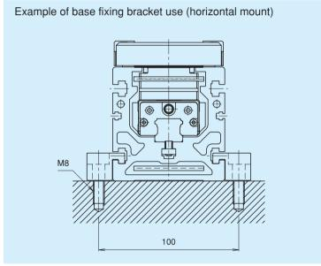
Note 1) Mounting position must be horizontal. If a wall mounting position is used, please contact THK. Note 2) Mounting intervals of the base fixing brackets should be approximately 250 to 300 mm.
