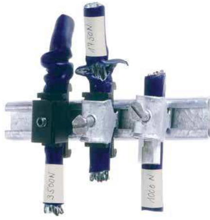
igus® test: Comparison of three different strain reliefs - Result: Triple tensile strength of igus® chainfix clamps compared to conventional products.
