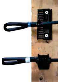
Tensile strength tests with chainflex® cables
