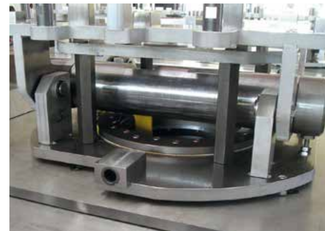
The lubrication-free iglidur® PRT slewing ring masters this job brilliantly, is lighter and in terms of purchasing is more affordable than a comparable metal rotary connector.
