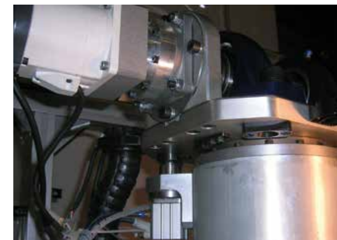
The iglidur® PRT-01-100 slewing ring is used in an automatic welding plant in this application. It enables pivoting in the horizontal plane of the clamping device.
