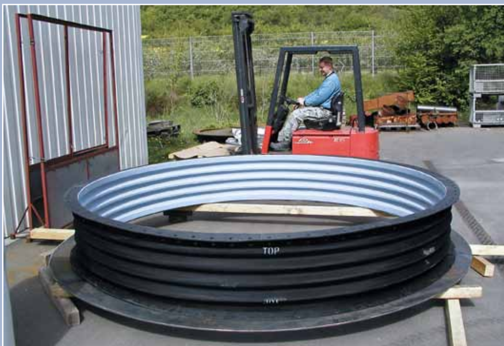
Universal expansion joint, type U142A with PTFE lining for a sulphuric acid reclamation plant NB 2800, -0.15 bar, 80 °C
