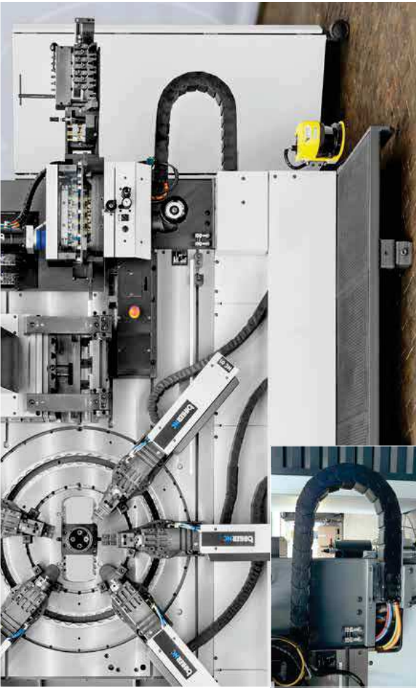
igus® R2.1 e-tube in operation in a fast stamping and bending machine to guide servo and encoder cables
