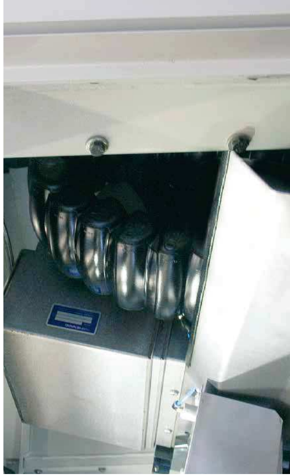
The RX e-tube used in this compact turning machine has Reverse Bend Radius ( RBR ) and operates even with the very restricted space
