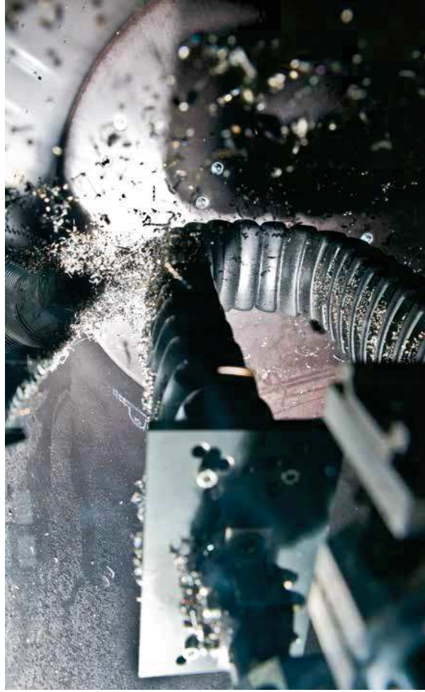
Swarf tests at the igus® test lab prove the excellent sealing of igus® RX e-tube. Video online ► www.igus.eu/RX_tested
