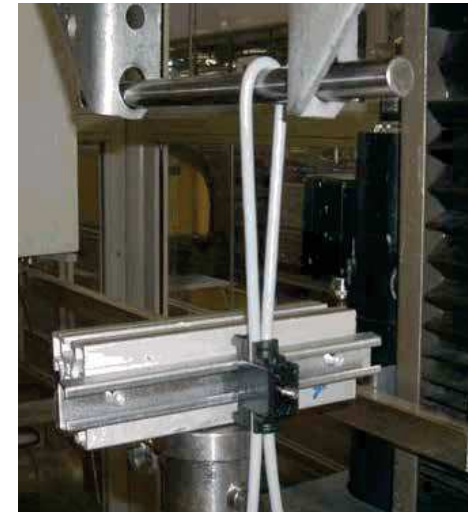
igus® tensile strength test CFX clamps with stacker saddle.
