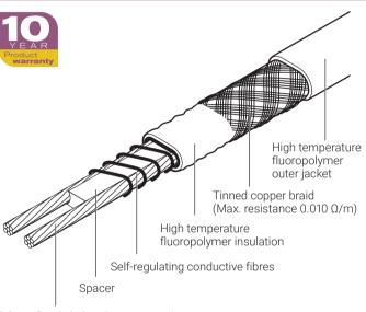
Electrical heat-tracing for process temperature maintenance applications up to 121°C which may be subject to steam cleaning.
