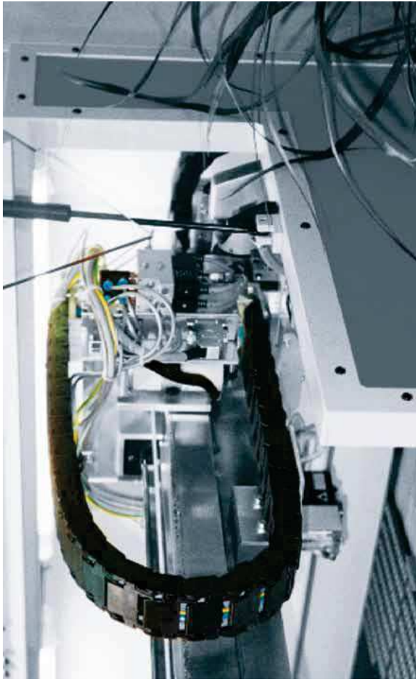
igus® zipper e-chain® series 15 in a special purpose machine for quick cable installation
